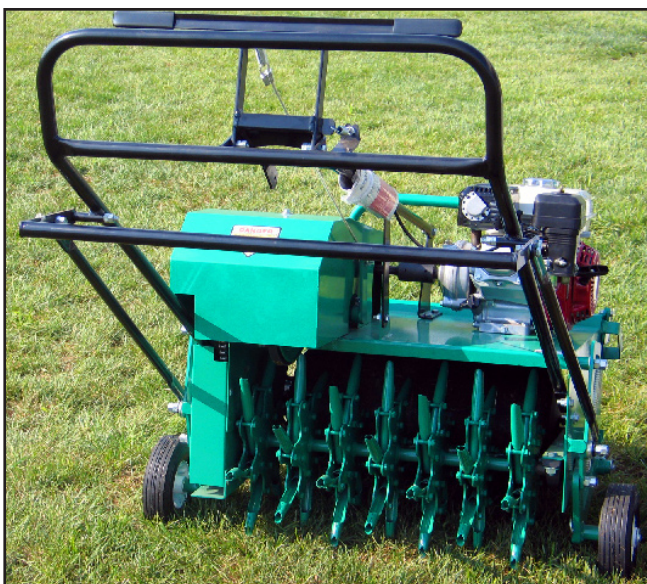
Figure 5. A walk-behind core aeration machine can be used on home lawns.
