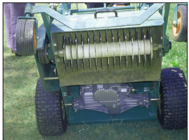
Figure 6. A vertical mower has blades that remove the thatch layer.
