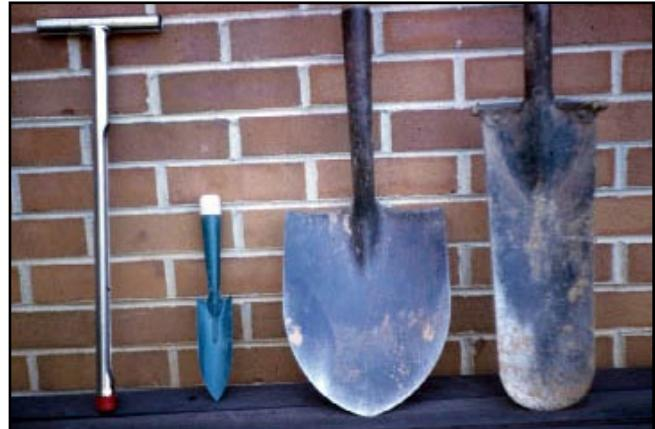
The soil probe is the best tool for collecting soil samples. The soil probe works better than a shovel or trowel because this tool equally collects soil in a continuous core from the surface through the entire sampling depth with minimal disturbance of the soil. It also allows for faster sampling.
